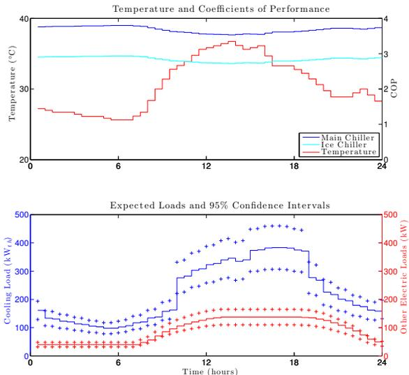
Fig. 2. Time-varying physical parameters. The top plot shows that the simulation day is particularly hot, with temperature peaking at 36.7 °C (98.1 °F). The coefficients of performance of both chillers decrease as the temperature increases, which encourages ice-making overnight. Note that the ice chiller is about 25% less efficient than the main chiller. The bottom plot uses two axes to distinguish thermal from electrical power.
