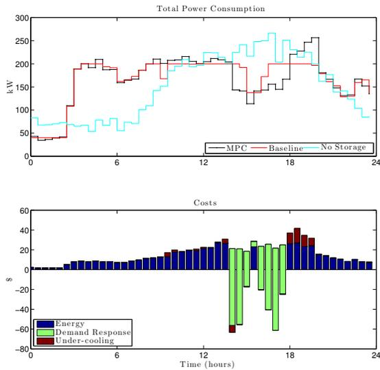
Fig. 4. Power and costs under the MPC policy. The baseline, shown in red in the top plot, is computed through OLOC with demand response prices set to zero. In the baseline calculation, the energy prices from 3-5 PM are high enough to shut down the main chiller. This low midday baseline significantly reduces revenues from the (overlapping) demand response event.
