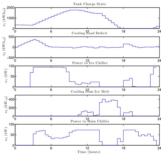
Fig. 3. States and controls under the MPC policy. Plots 2 and 5 show that the building is allowed to drift overnight when occupancy is low. Around 3 AM, both chillers turn on (plots 3 and 5) to fill the ice tank (plot 1) and cool the building back down (plot 2). During the demand response event (hours 14 to 18 in plots 3-5), both chillers are turned off and all cooling is provided by melting ice.
