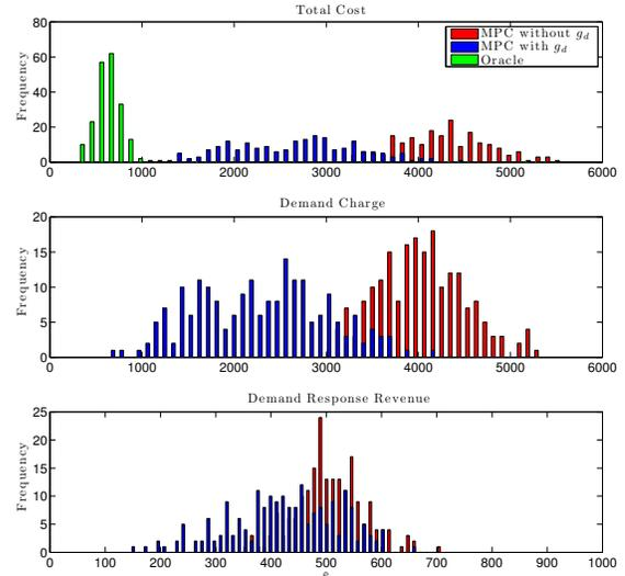
Fig. 5. Histograms of the total cost, demand charge and demand response revenues for 200 Monte Carlo runs. The average total cost of the oracle policy (\$630) is 23% that of the MPC policy (\$2,660). The MPC policy that neglects the demand charge incurs an average cost increase of 61% (\$1,610). In the absence of a demand charge, however, the average demand response revenue (and the corresponding energy reduction) increases by about 20% (\$80).
